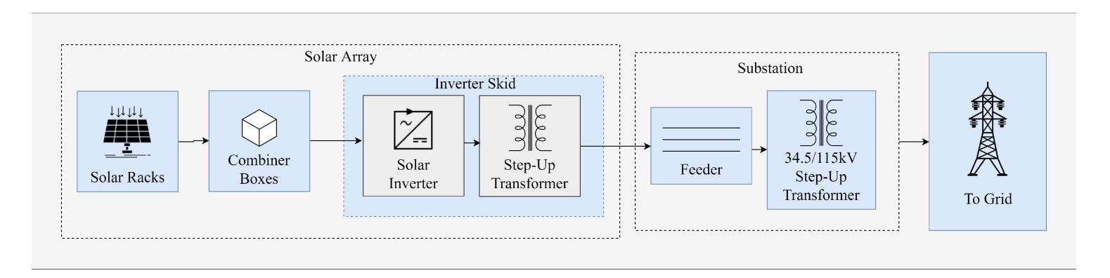
Below is a diagram showing how each inverter skid is connected to the substation through the feeders. Each inverter skid corresponds to one solar array. One collector contains three inverter skids.
